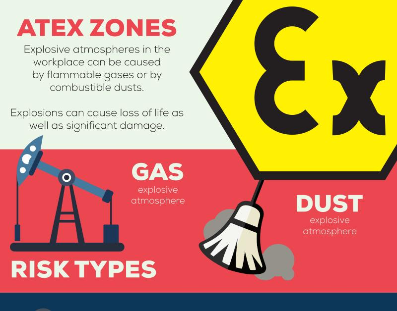
Three elements are required to cause an explosion: Fuel (gas or dust), Oxygen and an ignition source such as electric sparks or a short-circuit.
